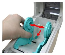
3. Feeds the media through the rear external label entrance chute. And place the paper, printing side face up, through the media guides, media sensor and place the label leading edge onto the platen roller.
