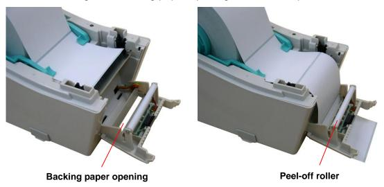
4. Push the peel-off panel back to the printer.
